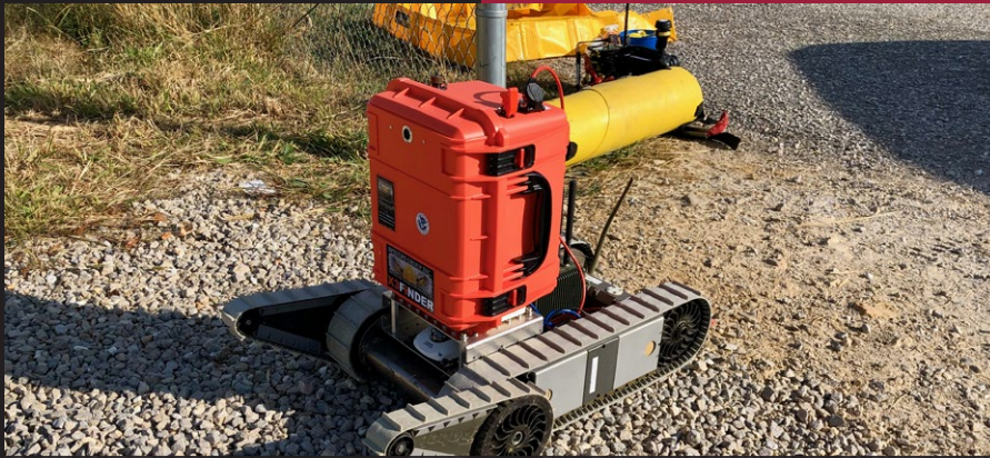
X3 Finder can also be mounted and configured to enable see-through-wall surveillance, enabling users to detect individuals within buildings, caves or tunnels
