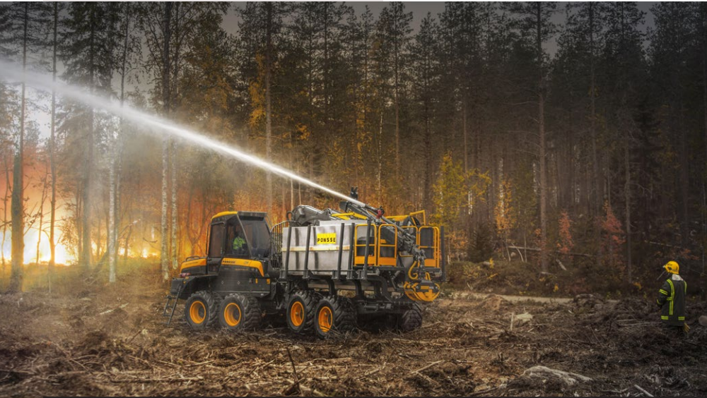
The Ponsse forwarder-mounted fire suppression system for rugged terrain
